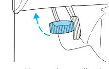
• Depress the clutch pedal (if equipped).
